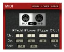
Here you select the channels for the three registers, adjust the octave position, and select keyboard splits, for playing more than one register on one keyboard.
