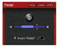
The minimum and maximum value can be set with the knobs A and B. The arrows show the actual position of the pedal. The pedal function can be inverted with knob C.
