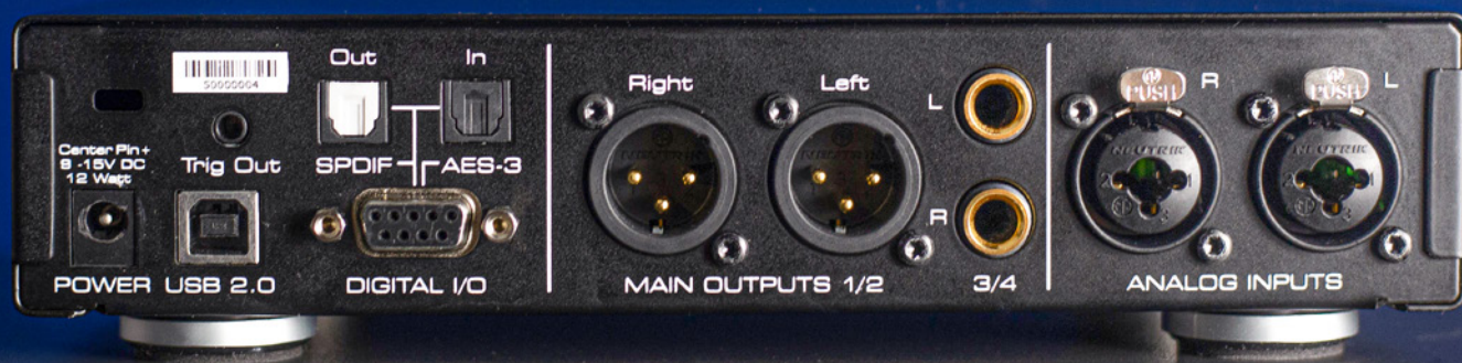
Round the back things are a bit busier, connection wise, with a 3.5mm trig output, USB B port, TosLink connectors and a D-type port for digital I/O, XLR and quarter-inch audio outputs and combi XLR audio inputs.
