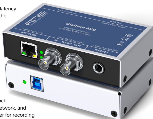
■ The Digiface AVB measures just 112 x 26 x 83 mm and includes an RJ45 port, a pair of BNC word-clock connectors, a headphone port and, round the back, a USB port for computer connection.
