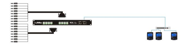
Using the Insert as Direct Out from Main Console to IEX-16L
