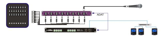
Using a audio from a DANTE Network via Rednet 3 Interface to IEX16L-A 32 input channels to myMix
