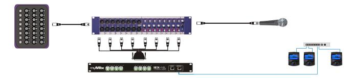
Using the Multicore Return for an Input from the Main Console to myMix
