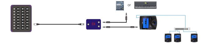
Splitting Microphone Signal for myMix and Main Console using a Mic Split Box
