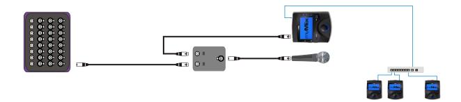
Splitting Microphone Signal using a central Microphone Split and IEX-16L with external Pre Amps
