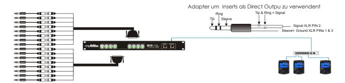
Using an Auxiliary Send from Main Console to IEX-16L
